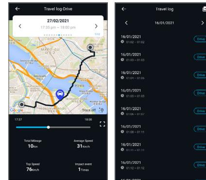
Travel-log-Drive shows vehicle's location on map, distance, speed, and event. You can check the data by date and time.
